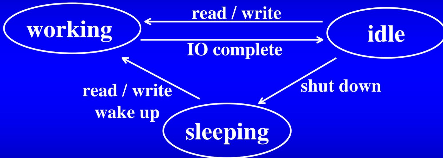
$$\text{Total Energy} = \text{time}_{\text{sleeping}} \times \text{Power}_{\text{sleeping}} + \text{time}_{\text{idle}} \times \text{Power}_{\text{idle}} + \# \text{ wakeups} \times \text{Energy}_{\text{wakeup}}$$
